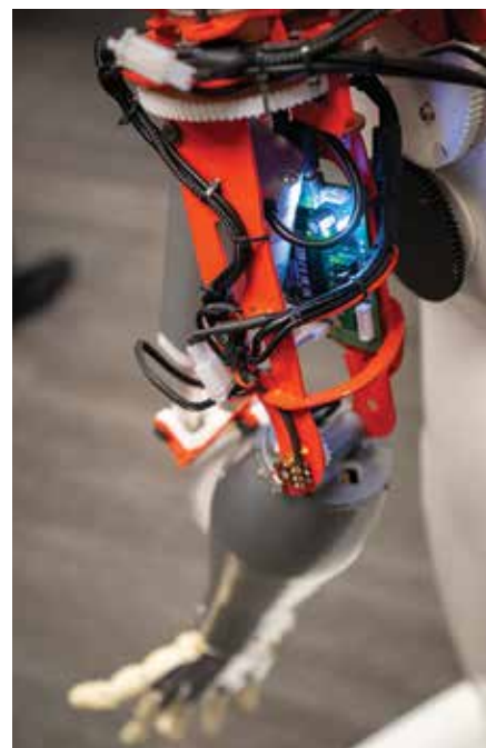
Mitra's hands use three types of motors for movement. The strongest motor, located at the shoulder, handles shoulder flexion and extension while a medium-torque motor at the elbow controls elbow movements. Five servo motors, one for each digit, are used to control the fingers.
